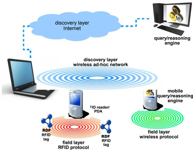
Figure 2. Field and Discovery layers in the *u-KB* framework architecture.
