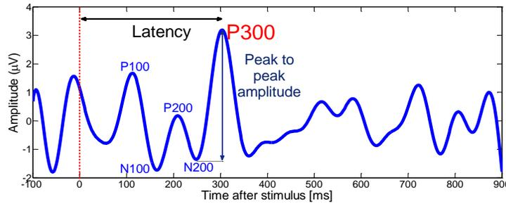
Fig. 1. Time-domain P300 waveform recorded on a healthy subject on a single EEG channel (PZ).
