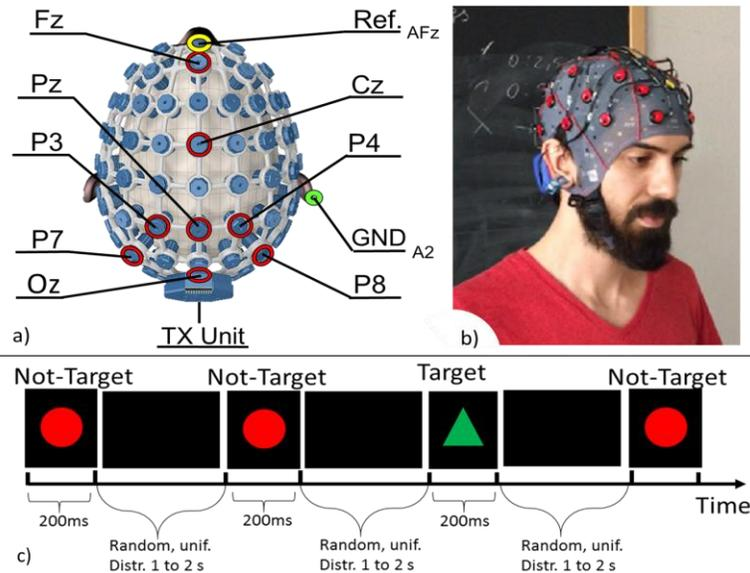
Fig. 3. a) Channels of interest (in red) according to the international system 10-20. In yellow the nasion reference and in green the ear-lobe ground. b) Demonstrative picture of the EEG wireless headset. c) time diagram of task A.
