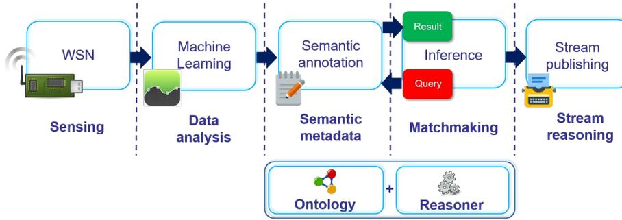
**Fig. 1.** Block diagram of the proposed approach for object (b)logging
