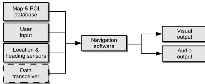
**Fig. 1.** General architecture of personal navigation systems
